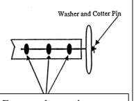
Fasten axle to axle support with J-bolts or Electrical Conduit Clamps so axle cannot turn.
